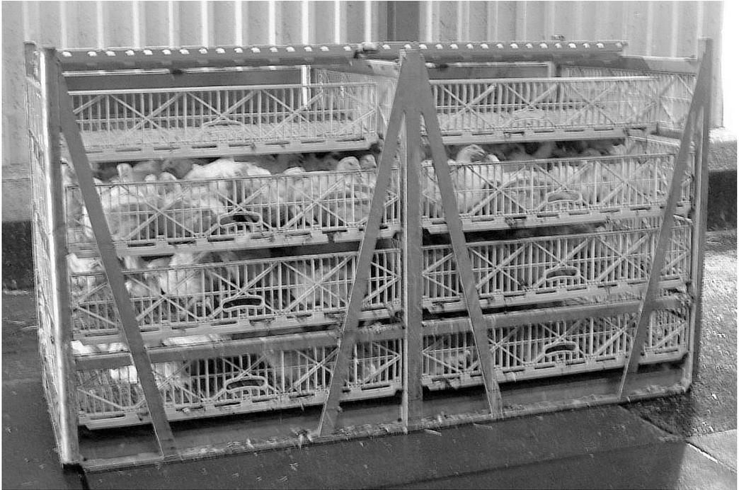
FIGURE 1. Live bird transport container; Stork GP container.
