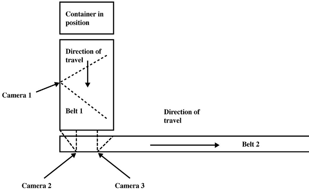
FIGURE 4. Schematic plan view of the camera positions in relation to major components.
