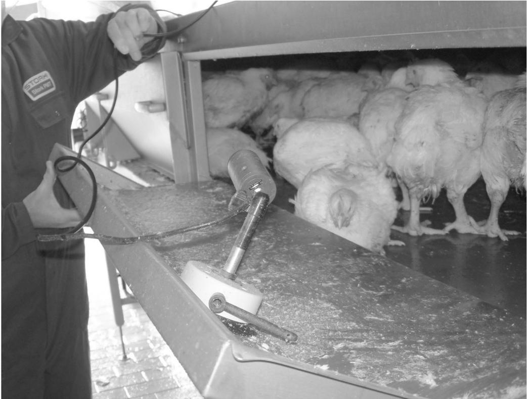
FIGURE 3. View through open hatch of pipe camera and vacuum clamp.
