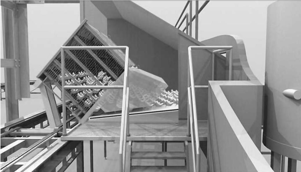
FIGURE 2. Cutaway view of automatic container handling system with container emptying.
